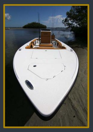
Bonefish boats are designed using a semi-monocoque technique to promote strength and rigidity, and are constructed from premium uv-resistant gelcoat, epoxy vinyl ester resin and high-density fiber-reinforced transom board.
